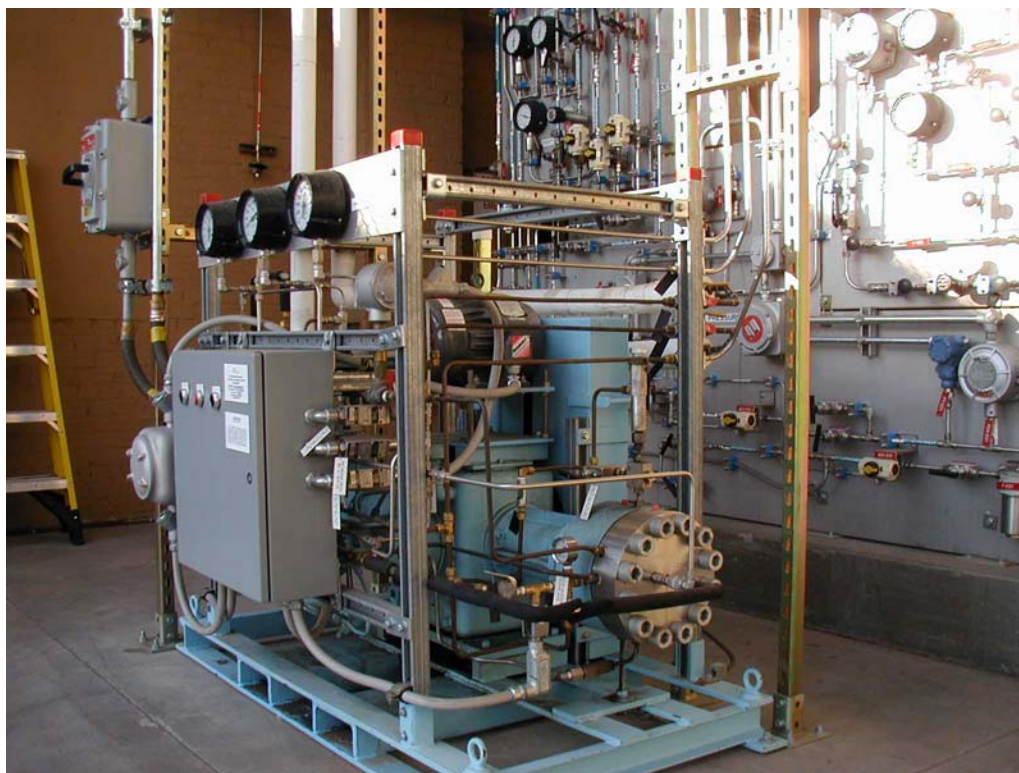
Figure 2.4. Pdc Machines, Inc. diaphragm hydrogen compressor.
